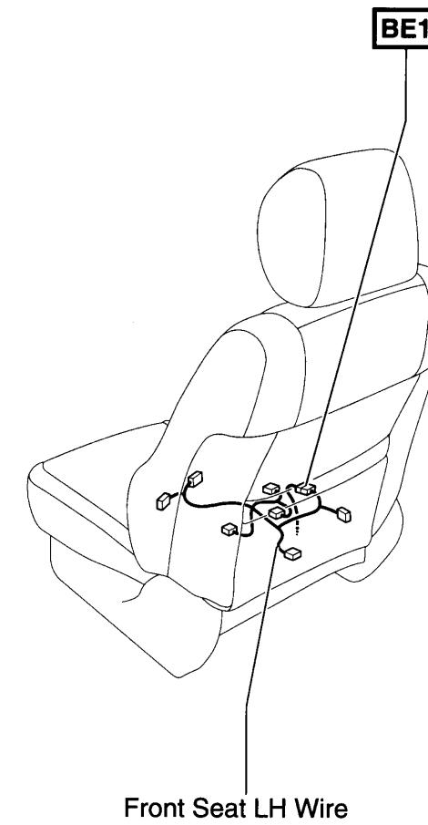
Connector Joining Wire Harness and Wire Harness
