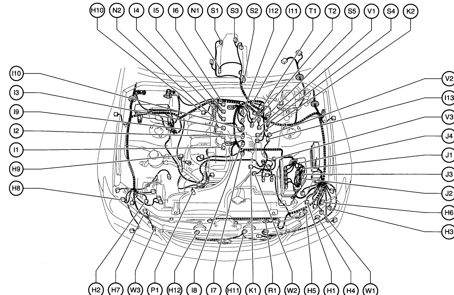
H 1 Headlight Beam Level Control Actuator LH
